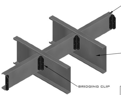
Rows of Joist Blocking Typically spaced at 2438mm (8') O.C. Along Joist Length.
