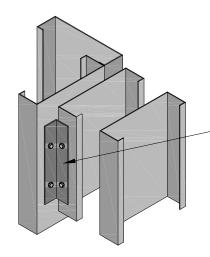
WHERE ACCESS TO CORNER IS LIMITED: CONNECT WALLS WITH BRIDGE CLIP VERTICALLY SPACED AND FASTENED WITH #10 SD/ST SCREWS
