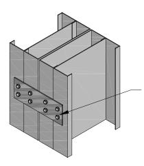
WHERE ACCESS TO CORNER IS LIMITED: CONNECT WALLS WITH FLAT STRAP VERTICALLY SPACED AND FASTENED WITH #10 SD/ST SCREWS
